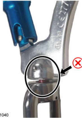
Fig 19. Red fall indicator exposed
